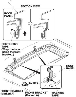
Using 3M protective tape application solution, spray the roof in the area shown where the moonroof visor will attach.
