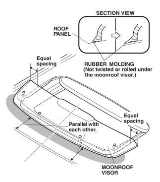
14. While holding the side brackets against the roof panel, tighten the two screws and nuts on the side bracket. While holding the front brackets against the roof panel, tighten the two screws and nuts on the front brackets. Using a torque screwdriver, torque all of screws to 2.0 N·m (1.5 lbf·ft).
