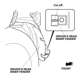
21. Install one spring nut over the hole in the driver's rear inner fender.
