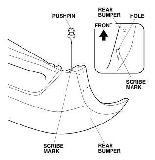
14. While wearing eye protection, drill a hole in the rear bumper with a 4 mm drill bit, then enlarge the hole with a 6 mm drill bit. Remove any burrs.
