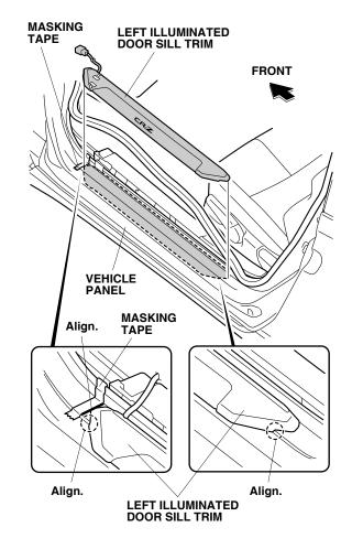
26. While applying light pressure against the left illuminated door sill trim, carefully remove the adhesive backings.
