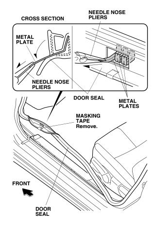
19. Remove the masking tape from the door seal.
