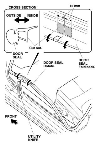
17. Using a utility knife, make a slit in the door seal at the location shown to expose the small metal plates inside the seal.
