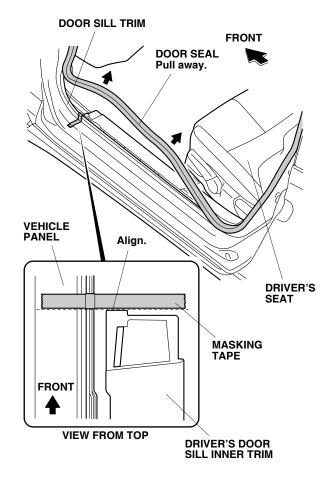
10. Attach a piece of masking tape to the vehicle panel. Align it with the front edge of the driver's door sill inner trim.  Align the left illuminated door sill trim with the masking tape.
