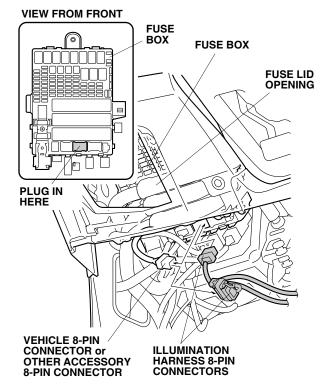
38. Plug the vehicle 8-pin connector into the illumination harness 8-pin connector. Go to step 41.
