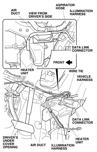
48. Secure the illumination harness to the vehicle harness with one wire tie.
