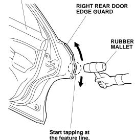
15. Repeat steps 3 through 14 to install the door edge guards on the left side of the vehicle.
