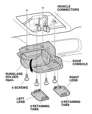
3. Remove the cover (two retaining tabs).
