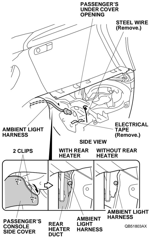
16. Route the ambient light harness as shown, then remove the electrical tape and steel wire.
