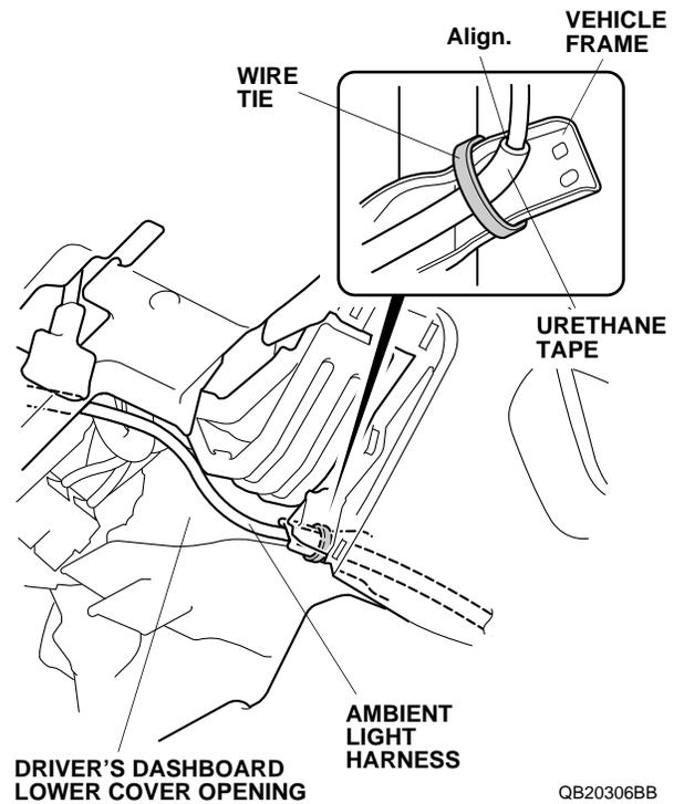
18. Secure the ambient light harness to the vehicle harness with one wire tie. Move the steering wheel up and down through its full adjustment range and make sure the harness is not being stretched.
