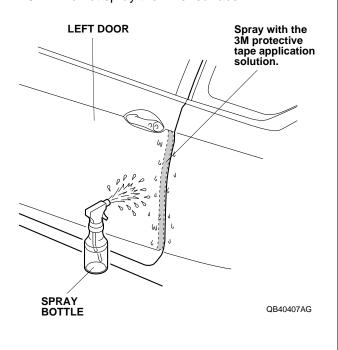
Open the left door. Peel back about 50 mm (2.0 in.) of adhesive backing from the left door edge film. Align the V-notch on the left door edge film 45 mm (1.8 in.) below the character line.
