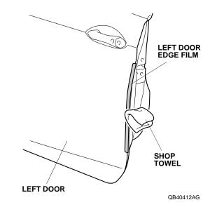
10. Repeat steps 1 through 9 to install the right door edge film on the right side of the vehicle.
