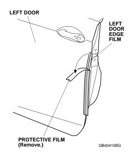
8. Starting from the center and working outward, use your finger to fold the left door edge film inside the left door. Move your finger in one direction only. Do not damage the door seam sealant.
