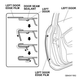
9. Using a shop towel, wipe the excess 3M protective tape application solution from the left door edge film. Allow the left door edge film to dry thoroughly.
