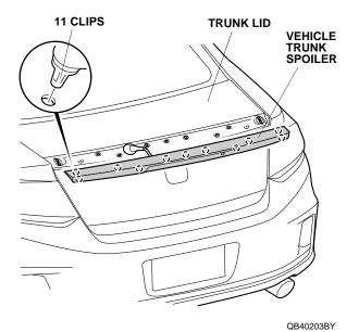
5. Cut the clip. Do not damage the vehicle harness.
