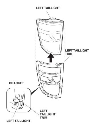
6. While holding light pressure on the trim, carefully remove all of the adhesive backings. After removing the adhesive backings, hold the trim firmly against the taillight with the palm of your hand for 30 seconds.
