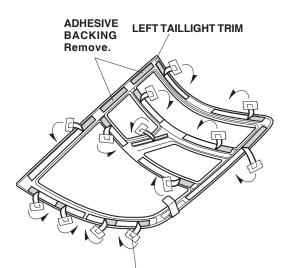
13 ADHESIVE BACKINGS Peel back 1½ to 2 in. [3-5 cm] of the adhesive backing strips and attach them to the front of the trim with masking tape.
