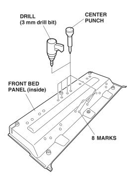
4. While wearing eye protection, enlarge the eight holes to 9 mm by drilling the outer surface of the front bed panel. Remove all burrs from the edges of the holes with a file.
