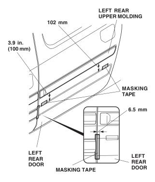
17. On the inside of the left rear lower molding, attach masking tape to the ends of the long adhesive backing and peel back 1½ to 2 in. (3-5 cm) from the adhesive backing. Tape the ends to the front of the moldings. Remove and discard all other adhesive backings.
