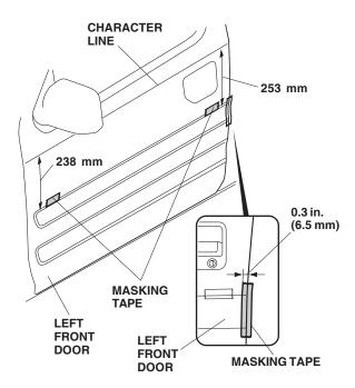
On the inside of the left front upper molding, attach masking tape to the ends of the long adhesive backing and peel back 1½ to 2 in. (3-5 cm) of the adhesive backing. Tape the ends to the front of the molding. Remove and discard all other adhesive backings.
