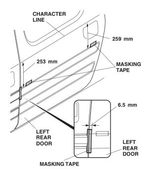
12. On the inside of the left rear upper molding, attach masking tape to the ends of the long adhesive backing and peel back 1½ to 2 in. (3-5 cm) from the adhesive backing. Tape the ends to the front of the molding. Remove and discard all other adhesive backings.
