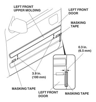
7. On the inside of the left front lower molding, attach masking tape to the ends of the long adhesive backing and peel back 1½ to 2 in. (3-5 cm) of the adhesive backing. Tape the ends to the front of the molding. Remove and discard all other adhesive backings.
