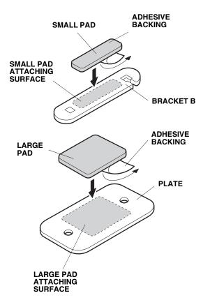
5. Using isopropyl alcohol on a shop towel, clean the four plates where the large pads will attach. Remove the adhesive backings from the large pads and attach them to the plates.
