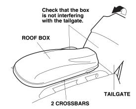
2. Open the roof box. Slide the plate forward or backward until the holes in the plate are over the front roof rack crossbar. The plate is located near the front of the roof box.
