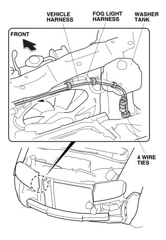
19. Secure the fog light harness to the vehicle harness using four wire ties.
