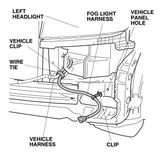
23. Secure the fog light harness to the vehicle harness using one wire tie.
