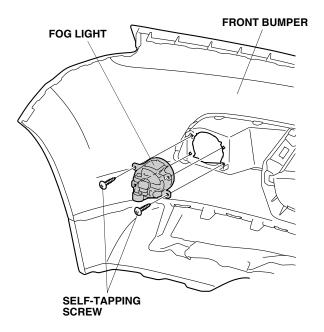
10. Reinstall the left fog light bezel to the front bumper.
