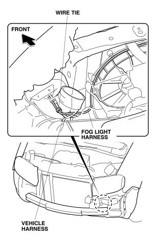
25. Secure the fog light harness to the vehicle harness using five wire ties in the areas shown.
