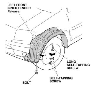
Insert your hand inside of the left front inner fender released in step 1. Unplug the connector from the fog light.
