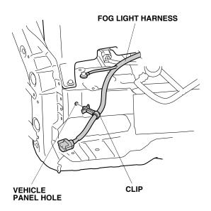
18. Route the other end of the fog light harness 2-pin connector up along the vehicle harness.
