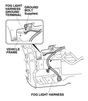
17. Secure the clip on the fog light harness to the vehicle panel hole.
