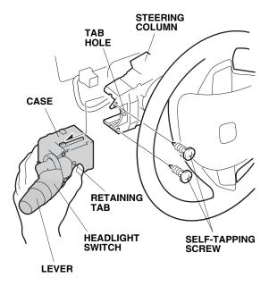
32. Install the new headlight switch to the steering column using two self-tapping screws. Hold the case by hand, then install the new headlight switch to the steering column.
