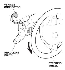
31. Remove two self-tapping screws from the headlight switch. While pushing the retaining tab, slide the headlight switch, and remove it from the steering column.
