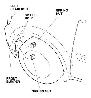
Check the position of the left front bumper trim and the left front fender trim to the front bumper and the left front fender. Remove the left front bumper trim and the left front fender trim.
