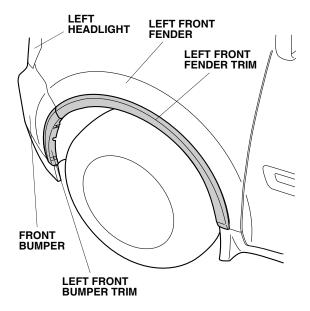
4. Using the alcohol swab, thoroughly clean the area where the left front bumper trim and the left front fender trim will attach.
