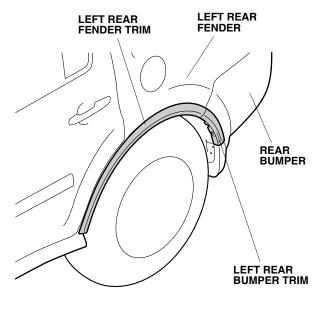
18. Using the alcohol swab, thoroughly clean the area where the left rear bumper trim and the left rear fender trim will attach.
