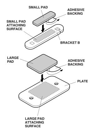
5. Using isopropyl alcohol on a shop towel, clean the four plates where the large pads will attach. Remove the adhesive backings from the large pads and attach them to the plates.
