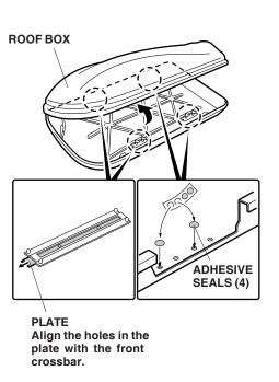
3. Attach adhesive seals over the unused rear mounting holes in the bottom of the roof box. The seals help prevent water from entering the roof box. Remove the roof box from the vehicle.
