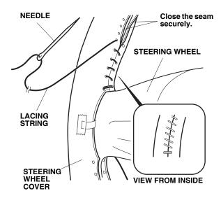
8. Keep lacing while adjusting the steering wheel cover so the seams on both sides of the steering wheel are aligned.
