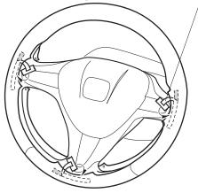
5. Thread the lacing string into the needle. Make inclined stitches in the back of the steering wheel cover up to the hole that is right above the spoke as shown.
