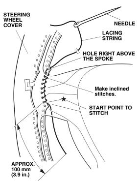
6. Lace twice through the hole right above the spoke, and pull the lacing string tight to close the seam.
