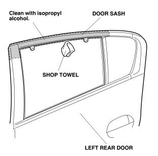
15. Remove the adhesive backing from the seal, and attach it to the door sash in the area shown.
