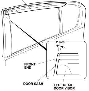
19. While holding the door visor firmly in position, remove the adhesive backing. Use your finger to push up each bracket so there is no gap between the brackets and the door sash.
