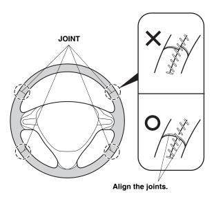
9. Stitch the spoke area of the steering wheel cover as shown. Stitch twice at the holes in the steering wheel cover that are right below and right above the spoke.
