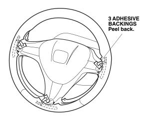
Thread the needle. Make inclined stitches in the steering wheel cover up to the hole that is right above the spoke as shown. Insert the needle into the hole in the steering wheel cover at the point marked below, and start stitching.
