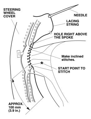
6. Stitch twice through the holes right above the spoke, and pull the lacing string to close the seam securely.
