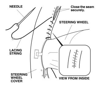
8. Keep stitching while adjusting the steering wheel cover so the joints on the cover are aligned.
