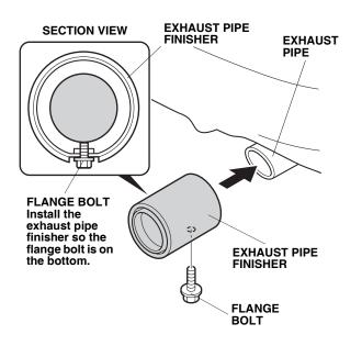
2. Slide the exhaust pipe trim firmly onto the exhaust pipe until it bottoms.
