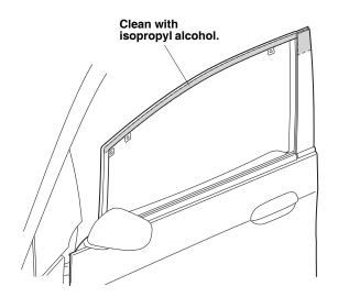
29. Remove the adhesive backing from a sealer, and attach it to the left front door as shown.
