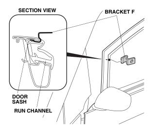
28. Using isopropyl alcohol, clean the door sash where the left front door visor will attach.
