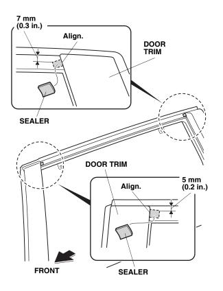
17. Peel back the adhesive backing partway and attach it to the outer surface of the left rear door visor with masking tape. Remove two adhesive backings.
