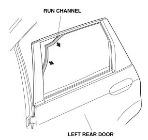
3. Open the run channel as shown, and measure where the EPT sealer (long) will attach.
