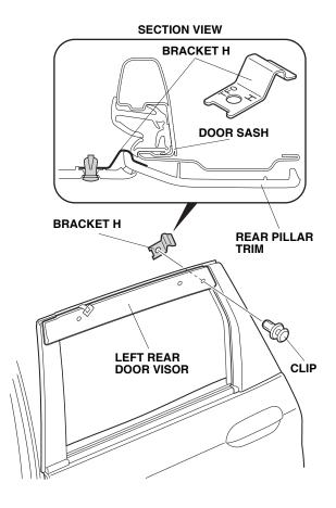
21. Remove the adhesive backing while pressing the left rear door visor in the direction of the arrow so there is no gap between the brackets and the door sash.
