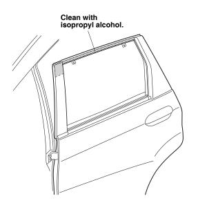
16. Remove the adhesive backing from two sealers, and attach them to the left rear door as shown.
