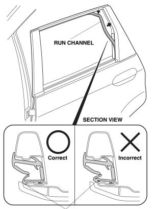
Check the run channel installation.
