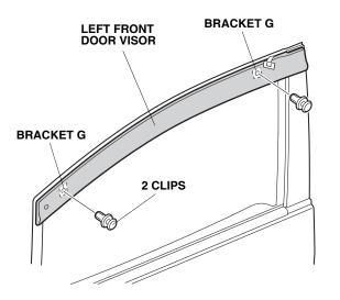
32. Push the left front door visor upward, and check that it aligns with the contour of the door trim. Push the brackets firmly against the door sash so there is no gap between the clips and the sash.
