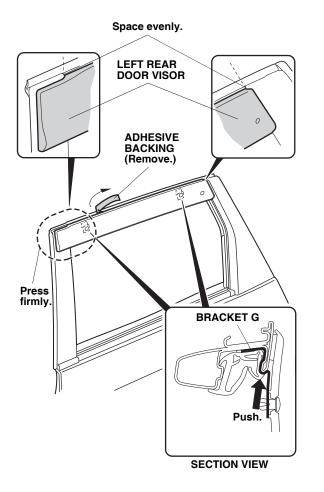
22. Press on the ends of the door visor for 30 seconds.
