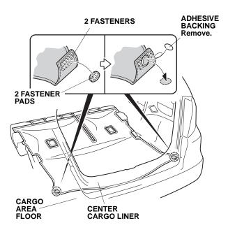
8. Remove the adhesive backings from the two fastener pads, position the center cargo liner, and attach the two fastener pads to the cargo area floor.
