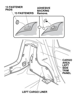
11. Remove the adhesive backings from the 13 fastener pads, position the left cargo liner, and attach the 13 fastener pads to the cargo area left side trim panel.
