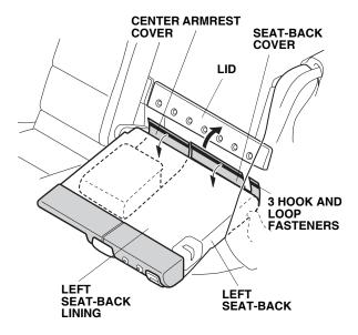
12. Repeat steps 7 thru 11 to install the seat-back cover on the right seat-back.
