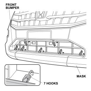
12. Route the elastic cord through the 13 loops on the bottom of the mask. Attach one hook to the hole in the inner fender. Stretch out the elastic cord after routing it through each loop, and then attach the other hook to the hole in the inner fender on the other side.
