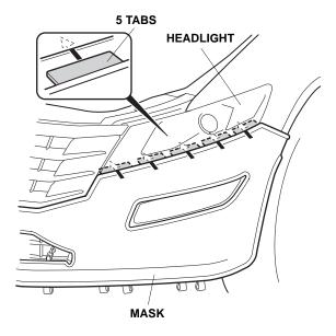
10. Insert the five center tabs between the front grille and the front bumper.
