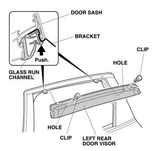
16. Align the door visor with the edge of the end cap.
