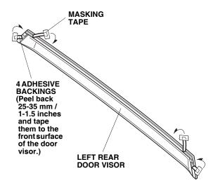
15. Align the clip holes in the visor with the bracket holes, and install two clips. There should be no clearance between the brackets and the door sash.
