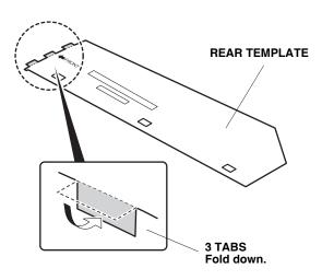
5. Insert the three tabs on the rear template around the front edge of the left rear door.
