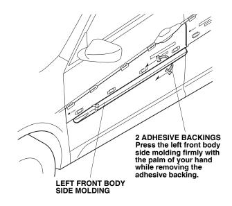
11. Using the rubber roller, apply firm pressure, especially at the ends, while rolling to set the adhesive.
