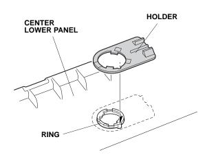
27. Secure the ambient light to the holder by rotating it into position. Go to step 34.
