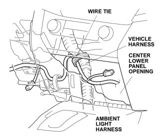
14. Continue routing the ambient light harness to the passenger's side of the vehicle as shown.
