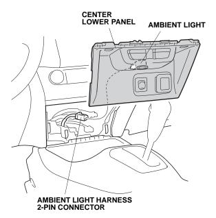
35. Install the ambient light to the right bracket by rotating it into position.
