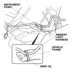
13. At the center lower panel opening, secure the ambient light harness to the vehicle harness with one wire tie.
