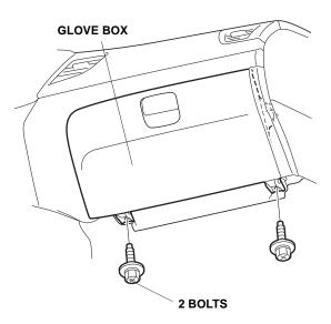
Open the glove box. Push inward on the stops, and remove the glove box.
