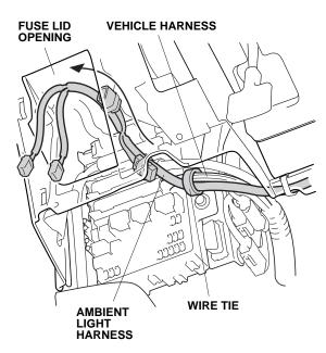
19. Using one wire tie, secure the ambient light harness to the vehicle harness.
