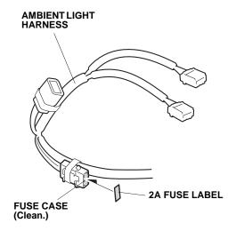
8. Attach the 2A fuse label to the fuse case on the ambient light harness.
