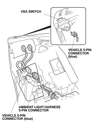
52. Plug the ambient light harness 5-pin connector (green) into the VSA switch.
