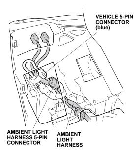
48. Plug the ambient light harness 5-pin connector (blue) into the ambient light switch, and plug the harness 5-pin connector (green) into the VSA switch.
