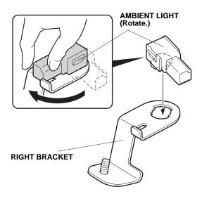
36. Plug the ambient light harness 2-pin connector into the ambient light.
