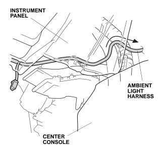
12. Using one wire tie, secure the ambient light harness to the vehicle frame.
