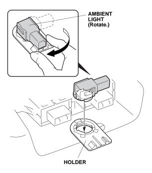
34. Plug the ambient light harness 2-pin connector into the ambient light, and reinstall the center lower panel.
