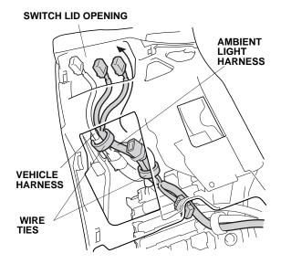
21. Using two wire ties, secure the ambient light harness to the vehicle harness.
