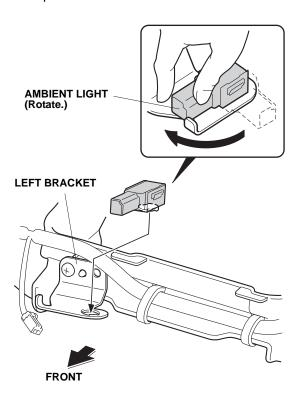
40. Plug the ambient light harness 2-pin connector into the ambient light.
