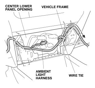
15. Using one wire tie, secure the ambient light harness to the vehicle frame.
