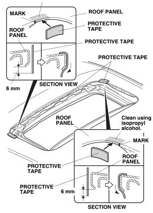
5. Remove the adhesive backings from two pieces of protective tape, and attach them to the roof panel at the two marks you made. Allow 6 mm of each protective tape to hang below the bottom lip of the roof panel. Remove the marks.  Locate the third indentations along the front edge of the moonroof opening. Using isopropyl alcohol on a shop towel, clean the roof area and the inside edge of the moonroof opening where the protective tapes will attach.
