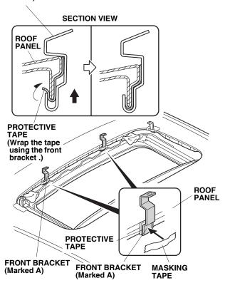
11. Set the moonroof visor on the vehicle roof in front of the moonroof opening, and adjust its position so the holes in the moonroof visor are aligned with the bracket holes. Loosely install the moonroof visor to the front brackets with two screws, two collars, and two nuts. Remove the masking tape.
