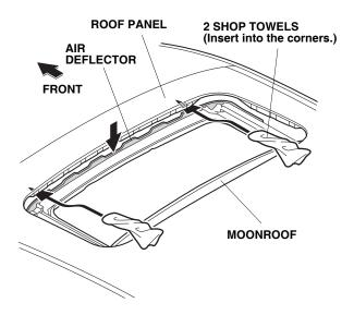
Locate the edge of the indentation on the right side and left side of the moonroof opening. Measure 45 mm to the front of the vehicle, and make two marks on the roof panel.
