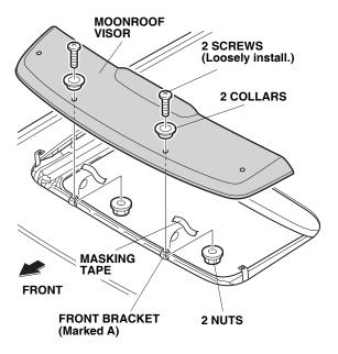
12. Loosely install the moonroof visor to the side brackets with two screws, two collars, and two nuts. Remove the masking tape.
