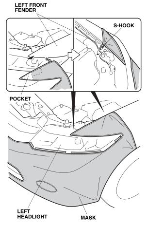
8. Attach the S-hook to the left front fender.
