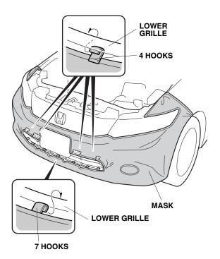
14. Insert four tabs between the bumper and the front grille.
