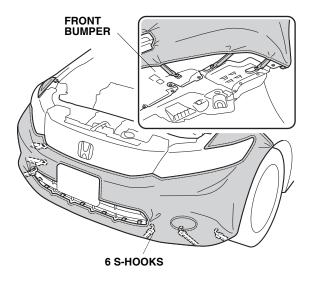
16. Route the elastic cord through the six loops on the bottom of the mask. Attach one S-hook to the bottom edge of the bumper on one side. Stretch out the cord after routing it through each loop, then attach the other S-hook to the bottom edge of the bumper on the other side.
