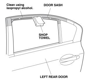
15. Remove the adhesive backing from seal A, and attach it to the door sash.
