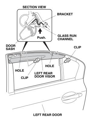
18. Adjust the left rear door visor to the position shown.
