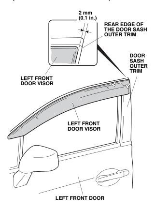
9. While applying light pressure against the left front door visor, carefully remove the adhesive backings. Use your finger to push up each bracket so there is no gap between the brackets and the door sash.
