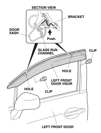
8. Adjust the left front door visor to the position shown.
