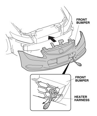
23. Using one black wire tie, secure the heater harness to the front bumper as shown.
