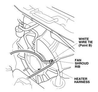
14. Route the heater harness up and toward the vehicle harness as shown.
