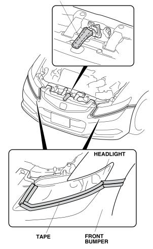
• Remove the 4 self-tapping screws, 10 short clips, and 2 long clips. Note the location of the long clips.
