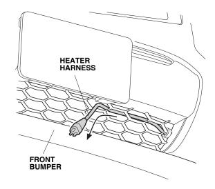
25. Using two black wire ties, secure the heater harness to the front grille as shown.
