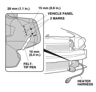
20. Using a pushpin, pierce the two marks on the vehicle panel. While wearing eye protection, drill the two pierced marks with a 3 mm drill bit, then enlarge the holes with a 5 mm drill bit. Remove any burrs.
