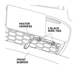
26. Attach the protective cap to the front grille, and plug the heater harness connector into the protective cap.
