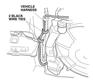
18. Route the heater harness through the front bulkhead as shown. Using one wire tie with clip, secure the heater harness to the vehicle frame.
