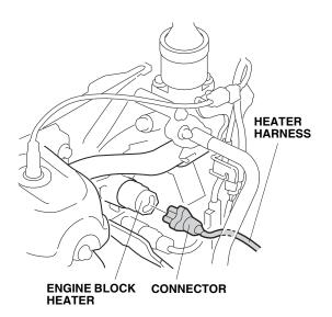
12. Secure the heater harness to the vehicle bracket with one white wire tie at the mark you made at point A.
