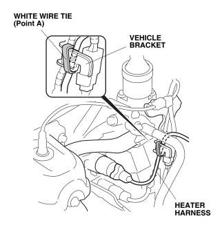
13. Route the heater harness along the fan shroud as shown. Secure the heater harness to the fan shroud rib with one white wire tie at the mark you made at point B.
