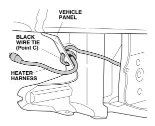
22. With the help of an assistant, route the heater harness through the grille opening in the bumper, then reinstall the front bumper with the help of an assistant.
