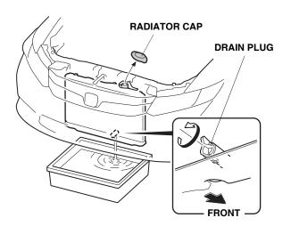
4. Drain the coolant completely, then reinstall the radiator cap.
