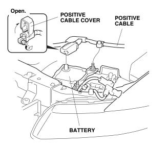
7. Remove the two nuts from the battery setting plate, and remove the battery setting plate and J-bolts. Remove the battery upper cover, battery, and battery under cover.
