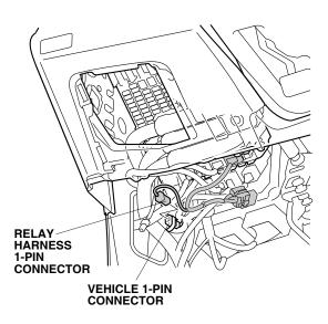
28. Remove the lower hood opener bolt. Secure the relay bracket to the vehicle panel with the hood opener bolt.
