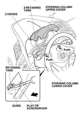
6. Remove the steering column upper cover (three retaining tabs and two hooks).
