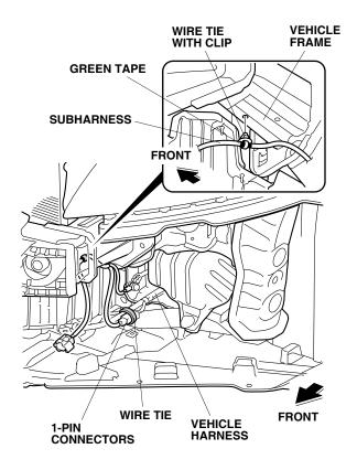
23. Secure the 1-pin connectors to the vehicle harness with one wire tie.
