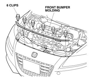
Remove ten clips, four self-tapping screws, and two washer-screws.
