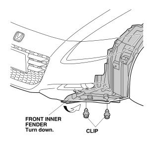
2. Insert your hand inside the inner fender. Unplug the connector from the fog light, and remove the bulb.
