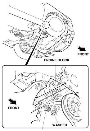
DRAIN BOLT Retain. Use a 19 mm socket. 11. Install the engine block heater with the aluminum washer into the bolt hole using a 24 mm socket and a torque wrench. Torque the engine block heater to 60 N·m (44 lbf·ft).
