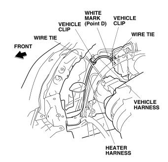
20. Route the heater harness forward, and secure it to the vehicle harness with one wire tie. Do not secure the heater harness to the SRS harness.
