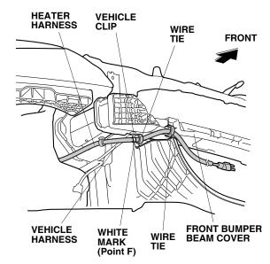
24. Secure the heater harness to the front bumper beam cover with one wire tie.
