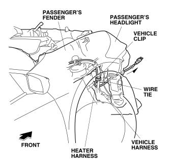
21. Route the heater harness along the front of the vehicle, and secure it to the vehicle frame with one wire tie with clip at point E.
