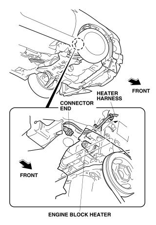
16. Route the heater harness along the engine block, and secure it to the engine block heater bracket with two wire ties with clips at point A and point B.
