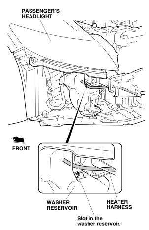
23. Align the white mark at point F to the vehicle clip on the front bumper beam cover. Secure the heater harness to the vehicle harness with one wire tie.
