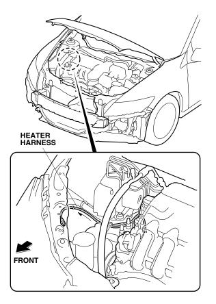
18. Secure the heater harness to the vehicle frame with one wire tie at point C.
