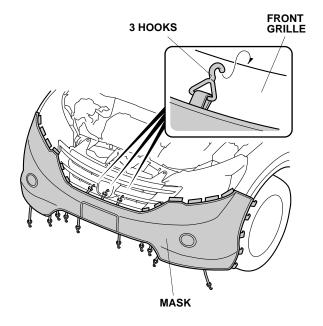
3. On each side, insert six tabs between the headlight/ grille and the bumper.
