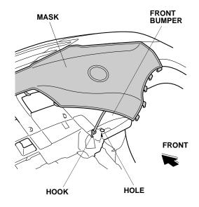
6. On each side, attach the five plastic hooks to the fenderwell.
