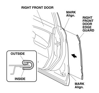
8. Starting at the feature line, tap the right front door edge guard into position with a series of light taps using a rubber mallet, then work up and down. Make sure the position of the right front door edge guard is correct. Once in place, do not remove, reposition, or reinstall the right front door edge guard.
