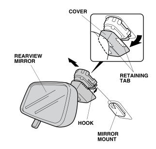
4. While holding down the hook, remove the rearview mirror from the mirror mount as shown.
