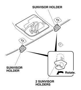
6. Rotate each sunvisor holders 45° counterclockwise to remove the two sunvisor holders.
