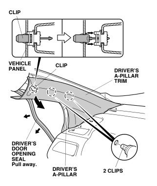
9. To prevent the clips from falling into the vehicle body, roll up the shop towel, and insert it between the driver's A-pillar and the dashboard. Take care not to damage the driver's A-pillar.
