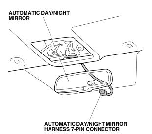
32. Route the automatic day/night mirror harness through the grooves in the harness cover. Secure the harness cover to the mirror stay as shown.
