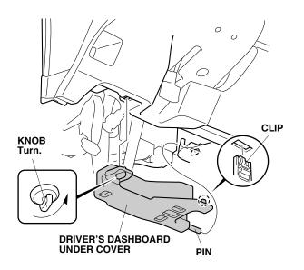
14. Remove the driver's dashboard lower cover (eight clips and unplug the vehicle connector).
