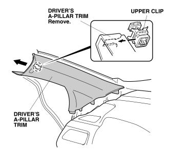
11. Remove the remaining upper clip from the driver's A-pillar.
