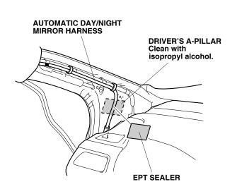
27. Gently pull down the headliner, and tuck the automatic day/night mirror harness under the headliner. Be careful not to crease the headliner.
