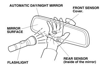
4. With the parking brake properly set, step on the brake pedal, and move the select lever to the "R" position. Repeat step 3, and check to make sure the mirror surface does not become dim. If the automatic day/night mirror does not function properly, check the fuse and all the connectors.
