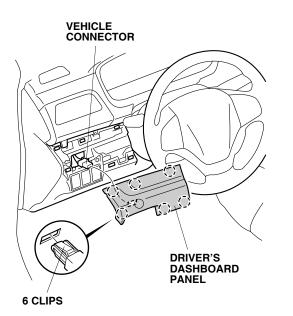
13. Remove the driver's dashboard under cover (turn the knob, one clip and one pin).
