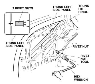
9. While holding the rivet tool with the hex wrench, turn the 27 mm wrench clockwise and install the rivet nut to the left trunk side panel.
