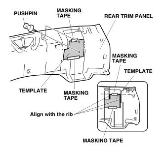
64. While wearing eye protection, drill a 3 mm hole at the four marked points, then finish with a 6.5 mm bit. Remove any burrs from the edges of the holes using a round file.
