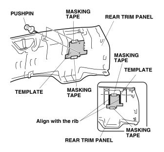
27. While wearing eye protection, drill a 3 mm hole at the four marked points, then finish with a 6.5 mm bit. Remove any burrs from the edges of the holes using a round file.
