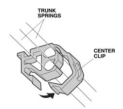
17. With an assistant holding the trunk lid open, use the trunk spring tool to remove the old trunk springs from the trunk hinge arms. Wear gloves to protect your hands, and pull the trunk spring tool slowly and carefully towards you.
