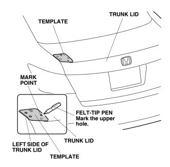
8. Flip the template over, and align it with the edge of the trunk lid on the right side. Using a felt-tip pen, make two marks on the right side trunk lid as shown on the template. Remove the template.
