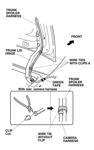
29. Route the trunk spoiler harness, and secure it to the vehicle panel holes with two wire ties with clips.
