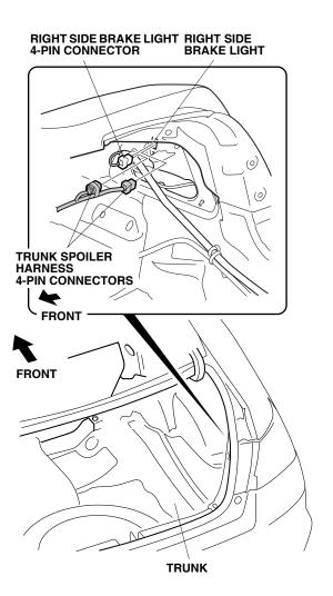
31. Plug the trunk spoiler harness 4-pin connector into the right side brake light. Plug the vehicle harness 4-pin connector into the trunk spoiler harness 4-pin connector.
