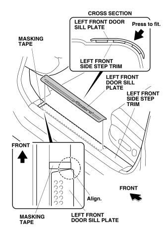
3. Using an alcohol swab, thoroughly clean the left front side step trim where the door sill trim will attach.
