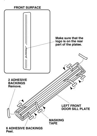
5. Align the left front door sill plate to the masking tape and press to fit the left front door sill plate to the left front side step trim as shown.
