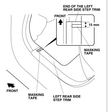
9. Align the front edge of the left rear door sill plate to the masking tape attached in step 8, then press on the left rear door sill plate to fit it to the left rear side step trim as shown.
