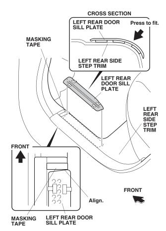
13. While applying light pressure against the left rear door sill plate, carefully remove the taped adhesive backings. Using the palm of your hand, firmly press the left rear door sill plate to the left rear side step trim.
