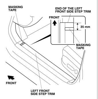
2. Align the front edge of the left front door sill plate to the masking tape attached in step 1, then press on the left front door sill plate to fit it to the left front side step trim as shown. Remove the door sill plate.
