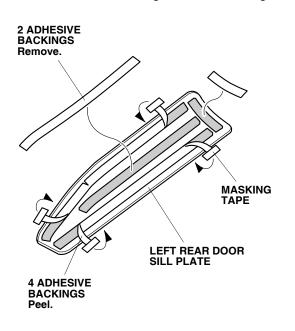
12. Align the left rear door sill plate to the masking tape and press on the edge to fit the left rear door sill plate to the left rear side step trim as shown.
