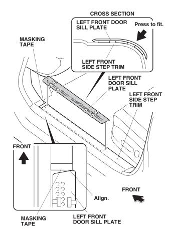
6. While applying light pressure against the left front door sill plate, carefully remove the taped adhesive backings in the order shown. Using the palm of your hand, firmly press the left front door sill plate to the left front side step trim.
