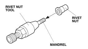
• Insert the rivet nut into the upper hole in the trunk left side panel, and install the hex wrench.
