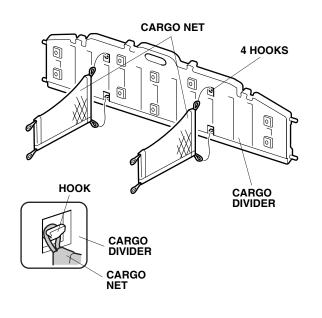
22. Slide the four pins on the cargo divider into the upright supports. Attach the cargo nets to the anchors on the rear trim panel. The cargo divider can be installed in two different positions:
