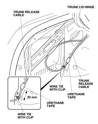
11. While wearing eye protection, enlarge the two clip holes to 10 mm:
