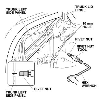
• While holding the tool with the hex wrench, use a 19 mm wrench to rotate the tool in a clockwise direction until the rivet nut is fully collapsed.
