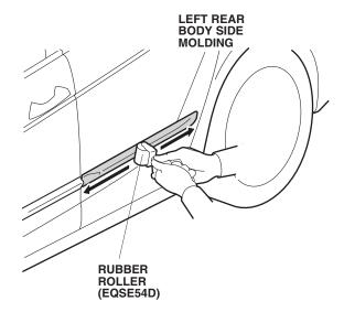
14. Turn the templates over and repeat steps 1 thru 13 to install the body side molding on the right side of the vehicle.
