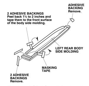
Align the end of the left rear body side molding with the rear template as shown and attach it at the front and back.
