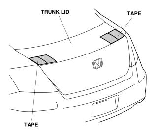
6. Align the template with the left side of the trunk lid. Using a felt-tip pen, mark the trunk lid as shown. Remove the template.
