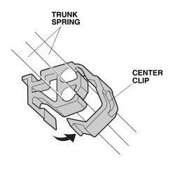
18. With an assistant holding the trunk lid open, remove the old trunk springs from the trunk hinge arms using the trunk spring tool. Wear gloves to protect your hands, and pull the trunk spring tool slowly and carefully toward you.
