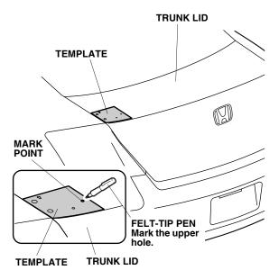
7. Flip the template over. Align the template with the right side of the trunk lid. Using a felt-tip pen, make two marks on the trunk lid as shown. Remove the template.
