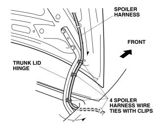
33. Route the spoiler harness. Secure the two spoiler harness wire ties with clips to the vehicle panel holes.
