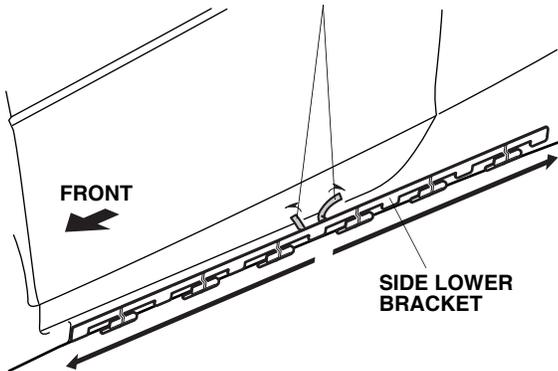
14. Attach the side lower bracket to the vehicle body by pressing it firmly with the palms of your hands or fingers where the double-sided adhesive tape is attached.
