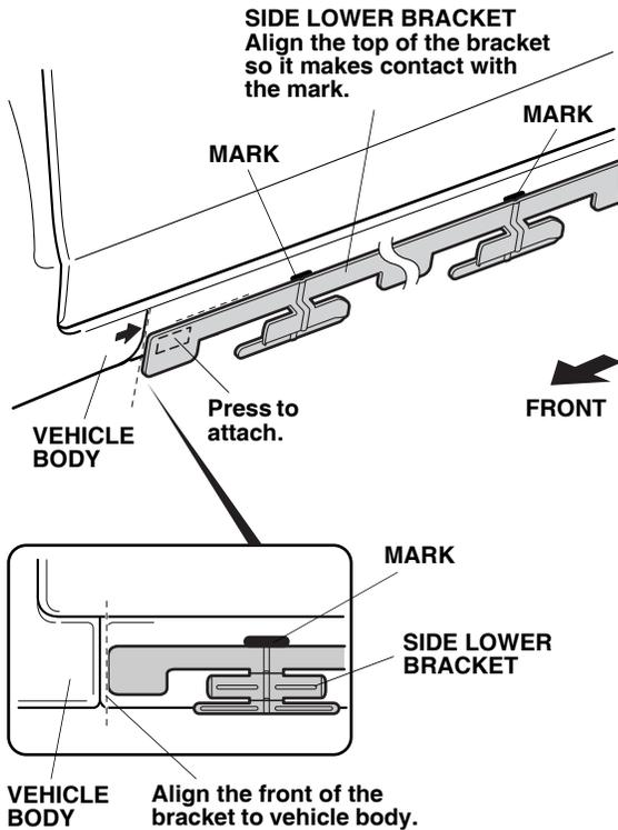
8. Raise the side lower bracket so that it makes contact with the marks.
