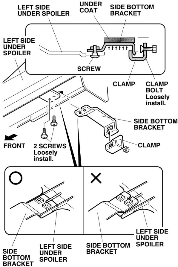
25. Remove the four adhesive backings from the left side under spoiler. Press firmly on the adhesive part of the left side under spoiler.
