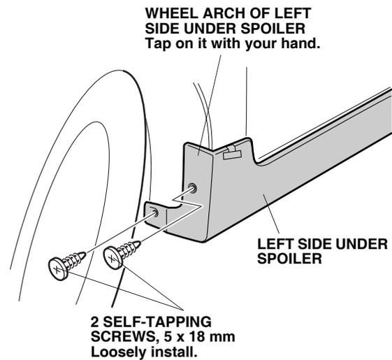
20. Check that all six brackets of the left side under spoiler are set in the side lower bracket installation plates. Visually check that there is no excessive gap between the left under spoiler and the vehicle. If an excessive gap is found, repeat step 19.
