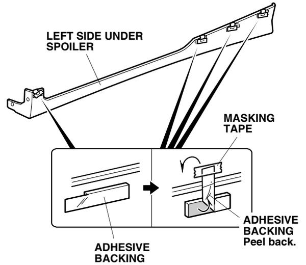
19. Check the position of the under spoiler attachments by looking down from the top. Slide the left side under spoiler rearward slightly while pushing it against the vehicle body with both hands.
