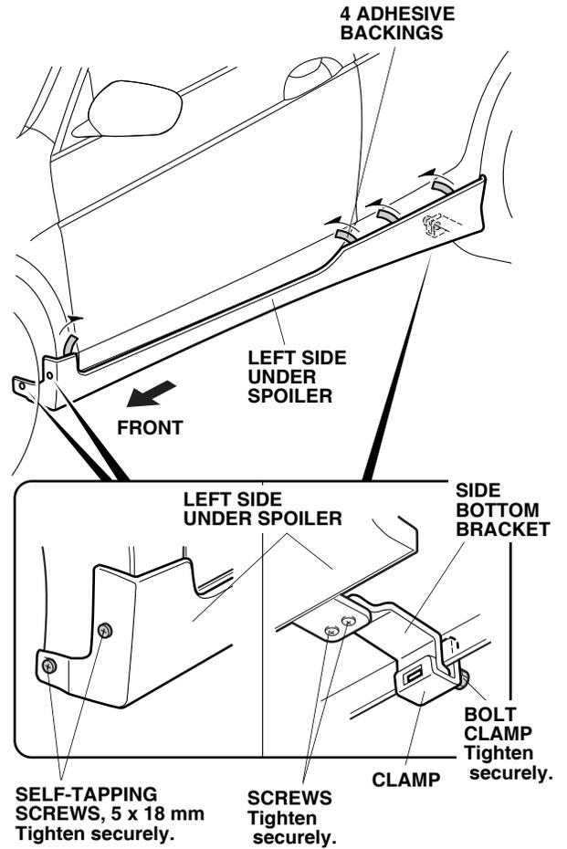
26. Tighten the two 5 x 18 mm self-tapping screws and the two screws securely.
