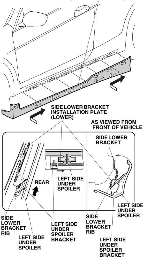
21. Gently tap on the left side under spoiler to remove any gap between the left side under spoiler and the left front inner fender.
