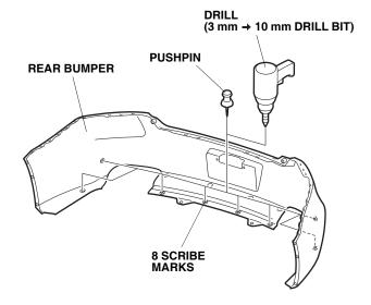
8. While wearing eye protection, first drill a 3 mm hole through the eight scribe marks from the inside of the rear bumper as shown. Finish with a 10 mm bit. Remove all burrs.
