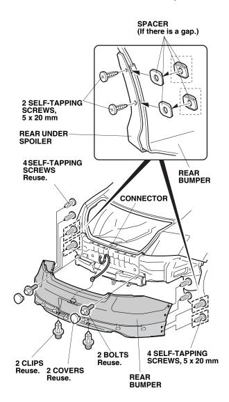
25. While applying pressure on the rear under spoiler, carefully remove the adhesive backings from the center outwards. After removing the adhesive backings, hold the rear under spoiler firmly against the rear bumper with the palm of your hand for 30 seconds. Apply pressure to the bumper from the inside and the outside with your hands as shown.
