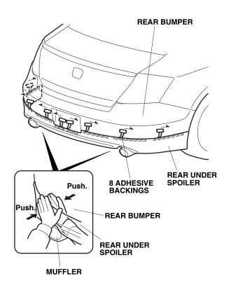
26. With a rubber roller, apply firm pressure while rolling to set the adhesive.
