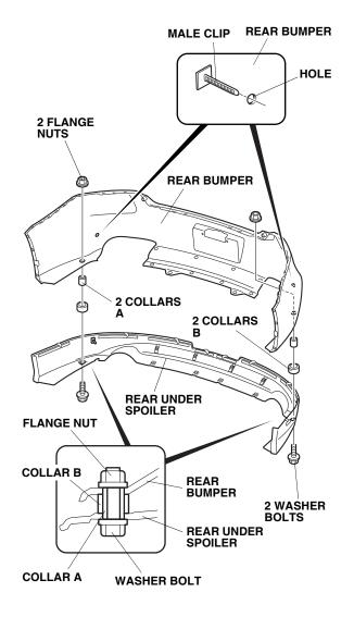
21. Secure the rear under spoiler to the rear bumper using four clips and two clip retainers as shown.
