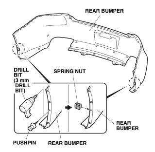
10. Slide two spring nuts over the two holes you made in the rear bumper.
