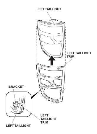
6. While holding light pressure on the trim, carefully remove all of the adhesive backings. After removing the adhesive backings, hold the trim firmly against the taillight with the palm of your hand for 30 seconds.
