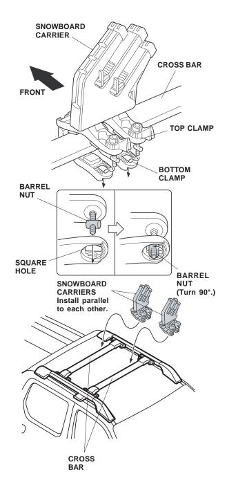
8. Turn the knobs on the top clamp to tighten the front carrier.
