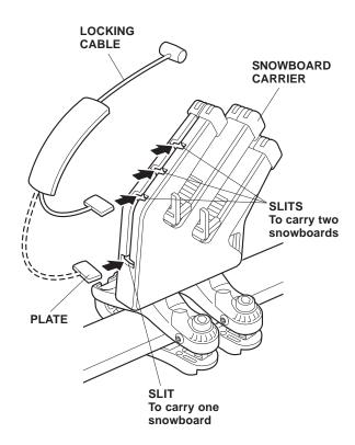
15. After loading the snowboard(s) on the carrier, adjust it (them) with the help of the board supports so that the top edges are level and the boards are as far down in the carrier as possible. To secure the snowboard(s) use the key to open the covers, and insert the locking cable stoppers into the holes of the carrier covers.
