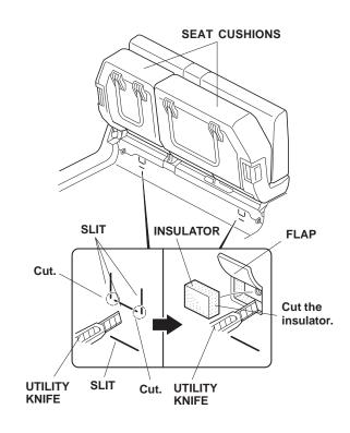
Lift the flap, and cut the insulator to locate the threaded hole.
