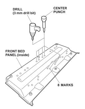
4. While wearing eye protection, enlarge the eight holes to 9 mm by drilling the outer surface of the front bed panel. Remove all burrs from the edges of the holes with a file.
