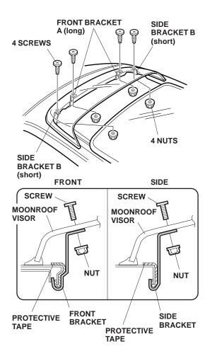
8. While holding the visor in place, install the brackets A and B with four screws and four nuts, with the end of each bracket hooked to the lip of the moonroof opening.
