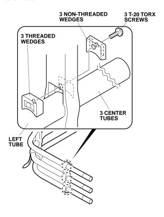
16. Insert three center tubes into the right tube (with label).
