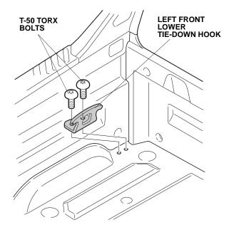
4. Reinstall the left front lower tie-down hook and the left bracket with two T-50 torx bolts (reused).
