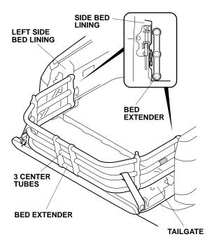
23. Align the non-threaded wedge with the threaded wedge at three joints between the right and center tubes, then secure the wedges with one T-20 torx screw each.
