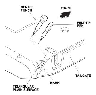
9. Using a center punch, mark the tailgate at the mark made in step 8.
