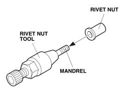
Insert the rivet nut into the rear under bumper and install the hex wrench on the rivet nut tool.
