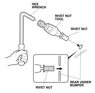
Holding the rivet nut tool with the hex wrench, turn the 19 mm wrench clockwise and install the rivet nut in the rear under bumper.
