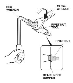
• Remove the rivet nut tool from the rivet nut by turning the hex wrench counterclockwise.
